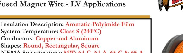
Shapes: Round, Rectangular, Square NEMA Specifications: MW: 64-C, 64-A, 65-C & 65-A Alconex Specifications: Alconex Aluminum and **Copper Specification**
